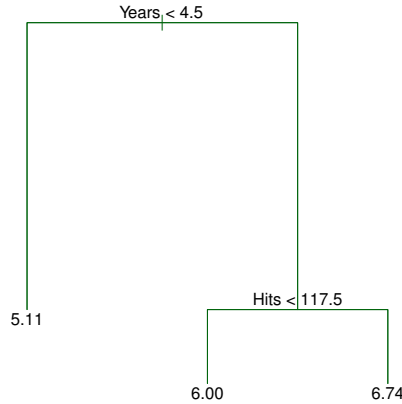
FIGURE 8.1. For the Hitters data, a regression tree for predicting the log salary of a baseball player, based on the number of years that he has played in the major leagues and the number of hits that he made in the previous year. At a given internal node, the label (of the form X_j < t_k ) indicates the left-hand branch emanating from that split, and the right-hand branch corresponds to X_j \geq t_k . For instance, the split at the top of the tree results in two large branches. The left-hand branch corresponds to Years <4.5 , and the right-hand branch corresponds to Years \geq 4.5 . The tree has two internal nodes and three terminal nodes, or leaves. The number in each leaf is the mean of the response for the observations that fall there.
