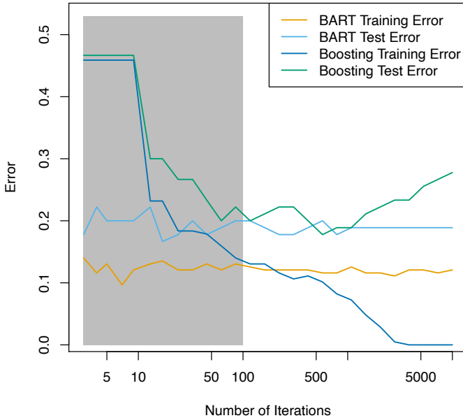
FIGURE 8.13. BART and boosting results for the Heart data. Both training and test errors are displayed. After a burn-in period of 100 iterations (shown in gray), the error rates for BART settle down. Boosting begins to overfit after a few hundred iterations.
